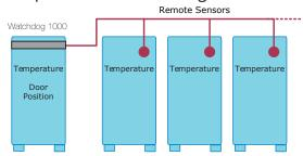
A single Watchdog 1000 with remote digital sensors, can monitor up to 17 cabinets. The total aggregate cable length for digital sensors may not exceed 600 feet.
