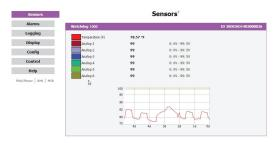
Readings from the internal temperature sensor and analog inputs are shown on the Sensors page.
